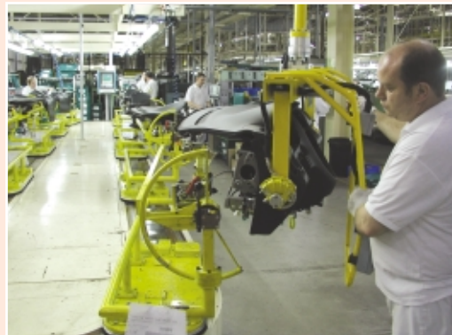
Instrument panel sub-assembly from Assembly Line 2
