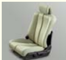
Seat made of new Honda bio-fabric
