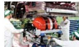
Installing the hydrogen tank
