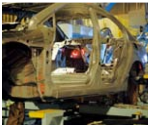
This high-precision automobile body process was achieved by introducing in-line measurement systems.
