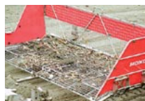
A sand rake picks up large refuse such as wooden fragments, netting, rope, etc., while a sand screen collects cigarette butts, glass shards, etc.
