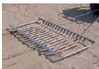
A sand rake picks up large refuse such as wooden fragments, netting, rope, etc., while a sand screen collects cigarette butts, glass shards, etc.
