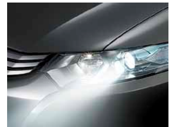
High-intensity discharge projector-beam headlights
