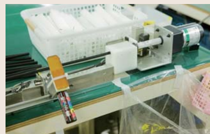
Karakuri -style innovation at work: A device that uses a store-bought pen to ensure that parts are marked properly for subsequent processing
