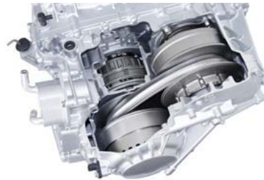
Honda's newly developed CVT for midsize vehicles
