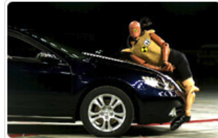
Collision testing with POLAR II at Honda's indoor omnidirectional Real World Crash Test Facility
