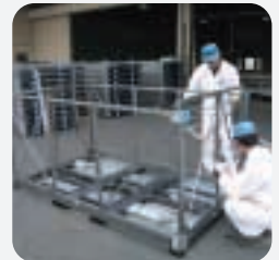
The new case can be easily assembled using square pipes and bolts.
