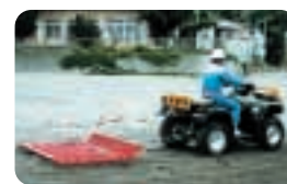
Extremely light beach cleaner to be pulled by an ATV
