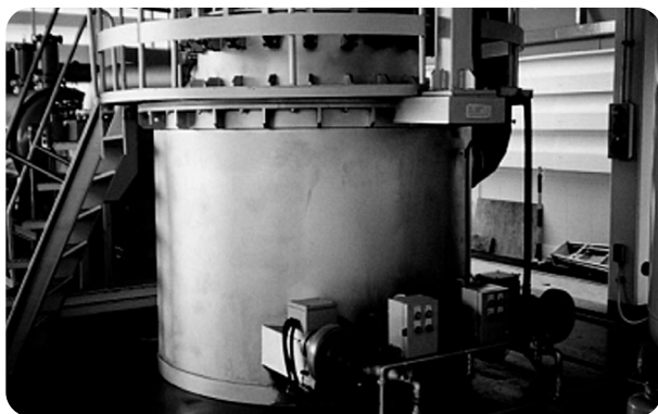
Dry distillation equipment for wastes
