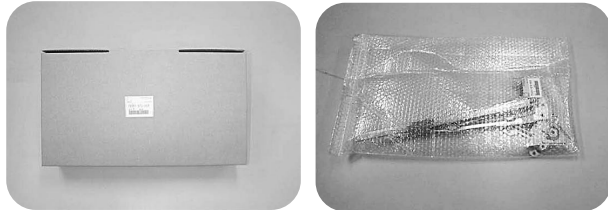
Before improvement (Individual packaging box) After improvement (Reinforced air cap)
