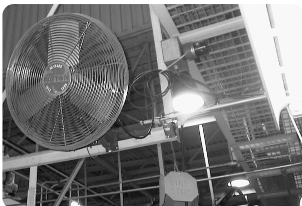
Automatically stopping fans for assembly line workers and sensors for this purpose
