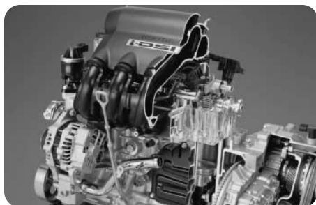
Section through the i-DSI engine
