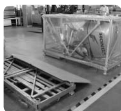
Returnable steel cases for outboard engines
