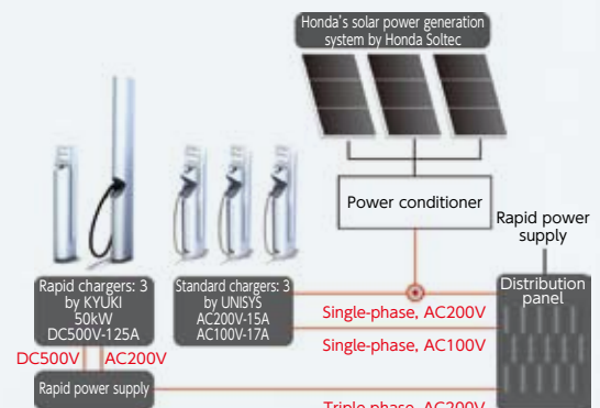
Concept for a solar charging station
