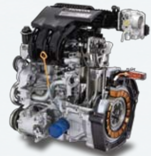
The Honda Hybrid System (1.3-liter i-VTEC engine + IMA)
