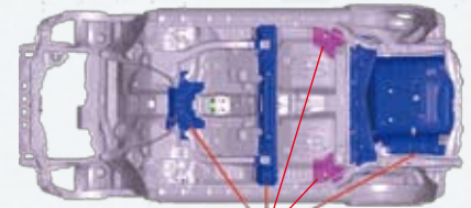
Body parts specially designed to accommodate IMA system
