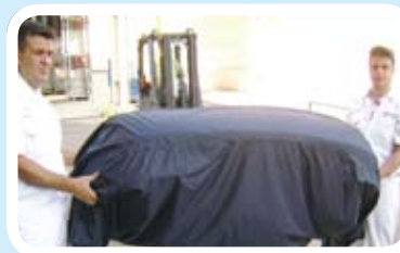
The nylon cover used for bumpers has been replaced with a reusable canvas.
