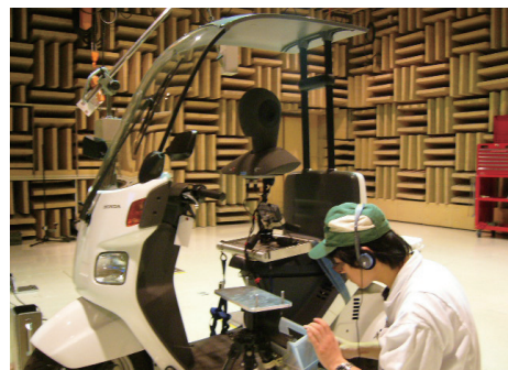
Sensitivity research using a dummy head microphone
