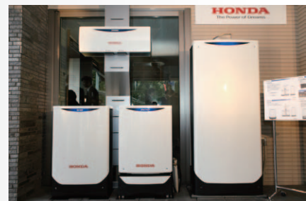
HSHS devices at the demonstration test home in Saitama (Smart e Mix Manager, gas-engine cogeneration unit, home battery unit)
