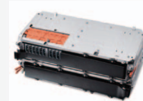
Left: Sport Hybrid i-MMD Plug-in lithium-ion battery (cut-away model) Right: Battery charger
