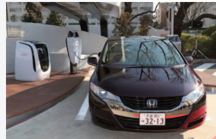
An FCX Clarity FCEV receives hydrogen from a solar hydrogen station installed at the south entrance to the Saitama Prefectural Office
