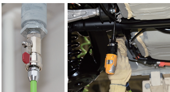
Leak-resistant hose joint (left) and assembly work using compressed air (right)
