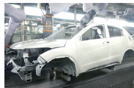
Honda S.E. Paint eliminated the need for a middle coat
