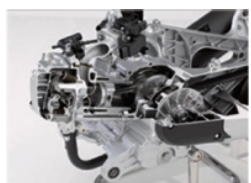
Global engine for next-generation compact scooters (cut-away model)
