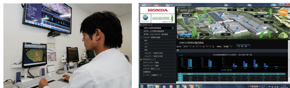
FEMS is used for centralized energy management of the entire plant (right: FEMS control screen)
