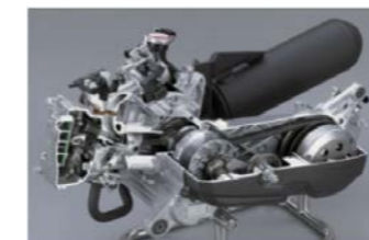
Newly developed eSP, a water-cooled, four-stroke overhead cam, single-cylinder 50-cc engine
