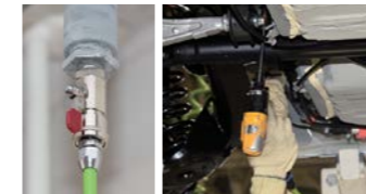
Leak-resistant hose joint (left) and assembly work using compressed air (right)
