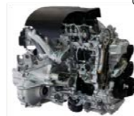
1.6-liter i-DTEC diesel engine (cut-away mode)
