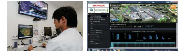
FEMS is used for centralized energy management of the entire plant (right: FEMS control screen)
